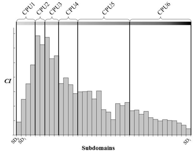
Figure 3: Conceptual illustration of load balancing. The cumulative computational intensity  $CI$  is evenly distributed among processors by assigning a varying number of subdomains.
